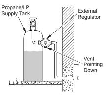
Figure 37 - External Regulator with Vent Pointing Down (Propane/LP Only)
